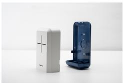
Optimized maintenance and calibration: one-step enclosure replacement
