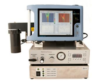
The LONESTAR device is used to separate most chemical compounds using FAIMS. Detected compounds can be visualised in real time using adapted software. All data can be immediately sent via Ethernet, USB, GPIO or wireless Bluetooth and then processed via remote control and analysis software. LONESTAR is a low-priced and easy to use product.
