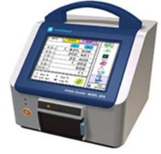
Compact and easy to use, the Particle Counter is available in two versions, the 3905 (flow rate 30lpm) and the 3910 (flow rate 50 lpm). These devices simultaneously measure and display the concentration of 6 different particle sizes: from 0.3 to 10  $\mu$ m. ISO 21501-4 compatible, the devices allow ISO 2 certification.
