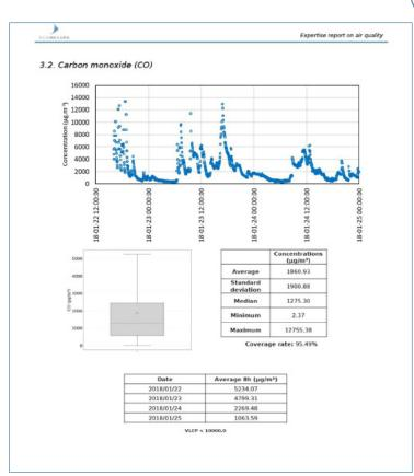
EcomReport is linked to the **Ecomzen** and **Ecomsmart** solutions, which are multiparameter, stations connected to the web platform, for monitoring air quality.
